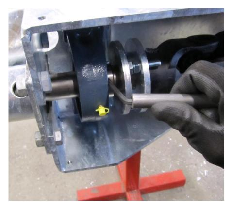
4. Adjust the distance in the pump housing by adjusting distance washers between the bearing and the universal joint. By reducing the distance between washers, the universal joint will be pushed down towards the bearing, and distance between the impeller and the cutter will decrease. It is important to check that the distance between the three adjustment screws is the same.
