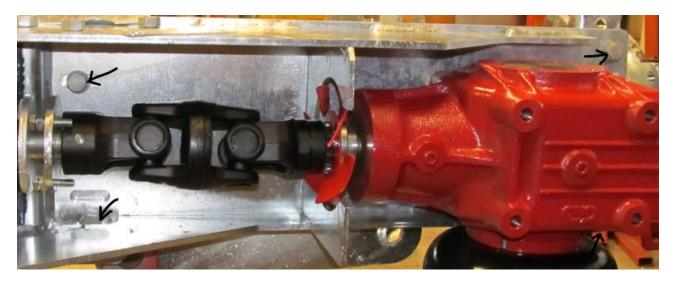
3. Release the set screws on the bearing.
