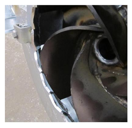
To maintain good cutting capacity, the distance between the impeller and the cutter must be 2-3mm. The distance is checked at least once per season or after 40 hours. If the distance is too small, a bump may occur which causes vibrations. Too large distance will result in a loss of power. The distance is adjusted as follows:
